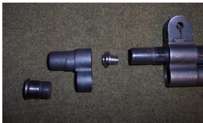
Fig. 3 Threaded “Hollywood” type blank firing adapter for M1 Garand
