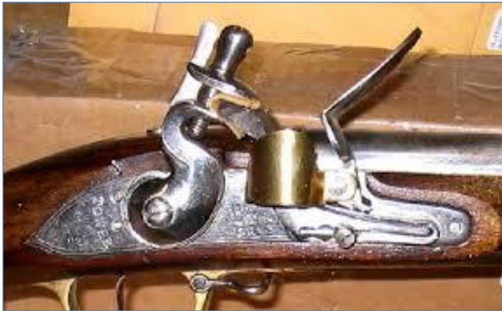
Fig. 1 Flash guard installed on reproduction Brown Bess musket
